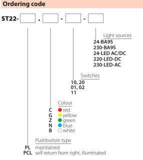
Description: the first digit represents the number of normally open circuits, the second digit represents the number of normally closed circuits.
