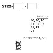
Description: the first digit represents the number of normally open circuits, the second digit represents the number of normally closed circuits. Letter A - the position in which the key can be pulled out Letter V - the position in which the key cannot be pulled out
