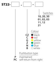
Description: the first digit represents the number of normally open circuits, the second digit represents the number of normally closed circuits.
